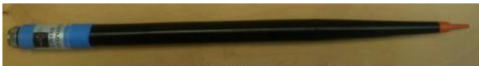
Figure 1 – MVG COMOSAR Dosimetric E-field Dipole
