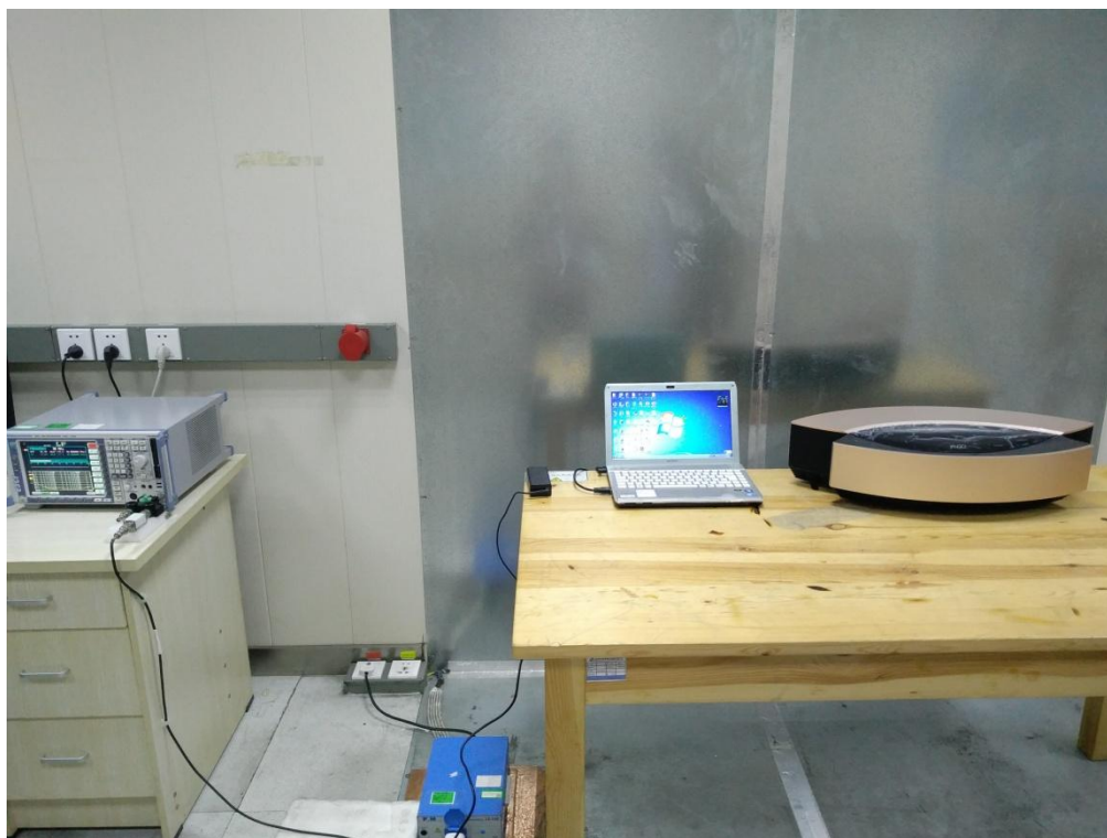
FCC RADIATED EMISSION TEST SETUP BELOW 1GHZ
