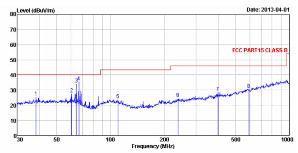
: 3m chamber : FCC PART15 CLASS B 3m VULB9163 -2012-05 HORIZONTAL Condition
