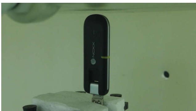
USB cable plug-in for Configuration 5 (Tip Side with Phantom 5mm Gap)
