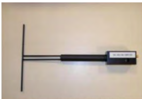
Figure 1 – Satimo COMOSAR Validation Dipole
