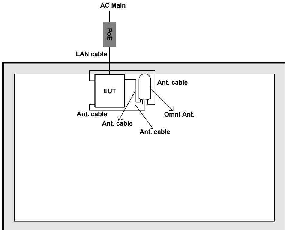
**Test Setup Diagram - Radiated Test - above 1GHz**
