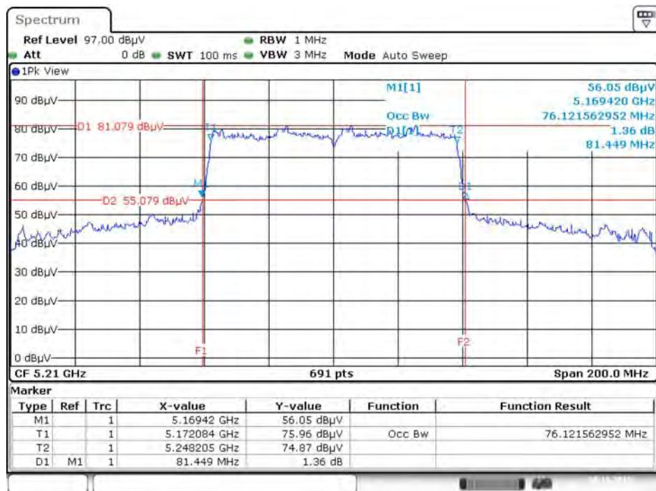
**26dB Bandwidth and 99% Occupied Bandwidth Plot on Configuration IEEE 802.11ac MCS0/Nss1 VHT80 / Chain 5 + Chain 6 + Chain 7 + Chain 8 / 5775 MHz**
