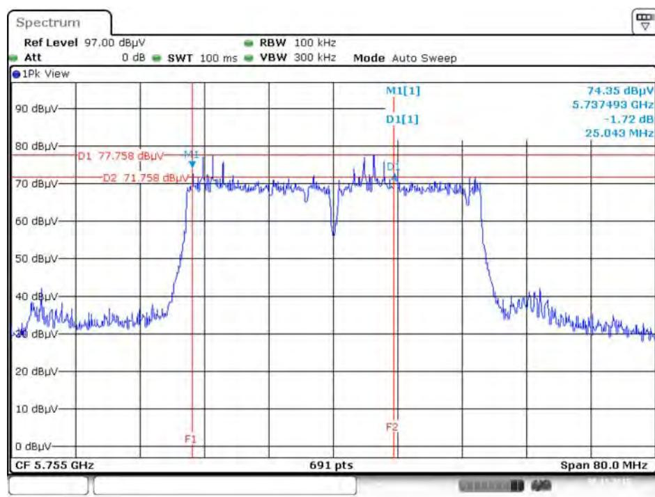
**6 dB Bandwidth Plot on Configuration IEEE 802.11ac MCS0/Nss1 VHT80 / Chain 5 + Chain 6 + Chain 7 + Chain 8 / 5775 MHz**
