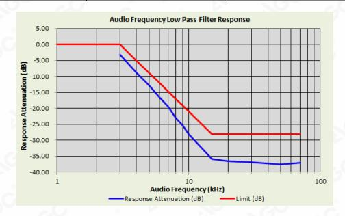
Note: All the test frequencies was tested, but only the worst data be recorded in this part.
