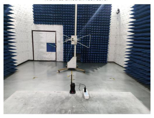
RADIATED EMISSION ABOVE 1G TEST SETUP
