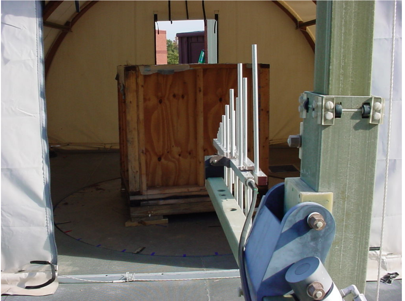
Figure 7: Test Setup Radiated Emissions - Intentional
