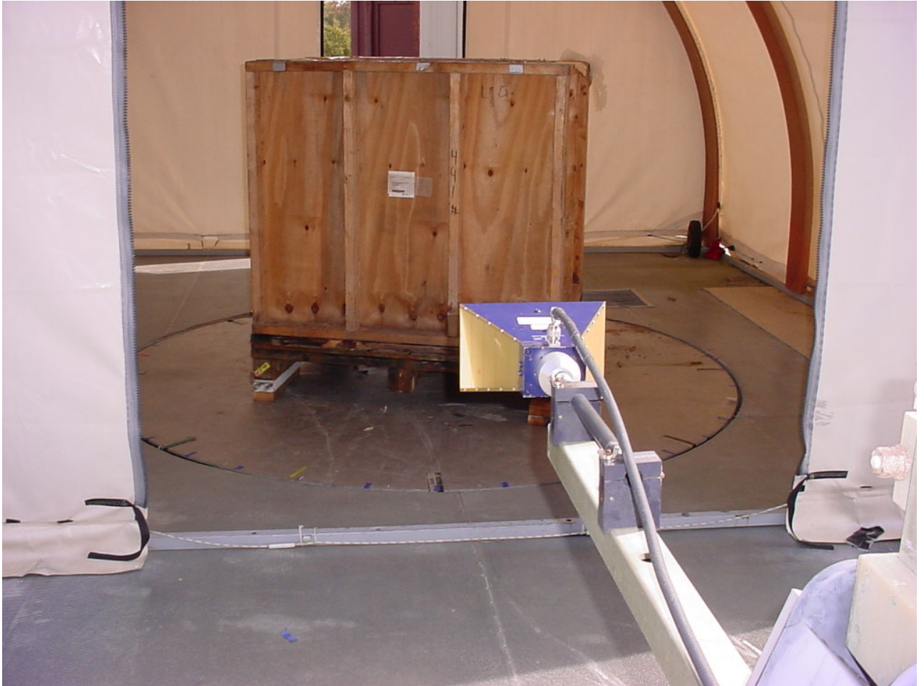
Figure 5: Test Setup Radiated Emissions - Intentional
