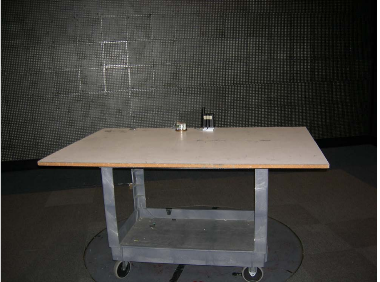
Figure 2: Test Setup Radiated Emissions - Unintentional
