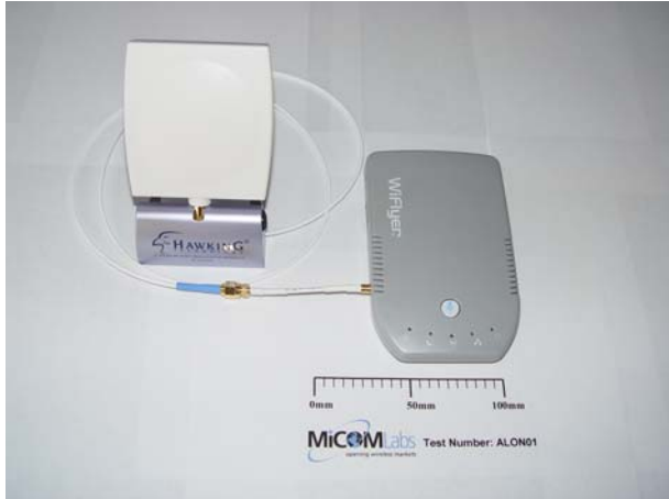
WiFlyer with Hawkins 6dBi Omni Directional Antenna
