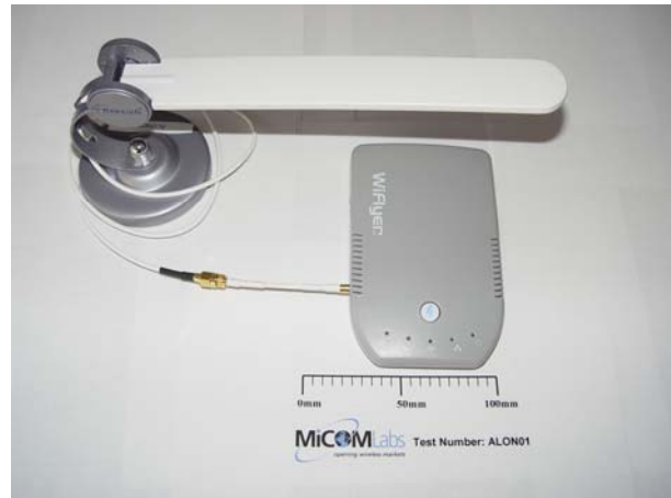
WiFlyer with Hawkins 6dBi Dipole Antenna
