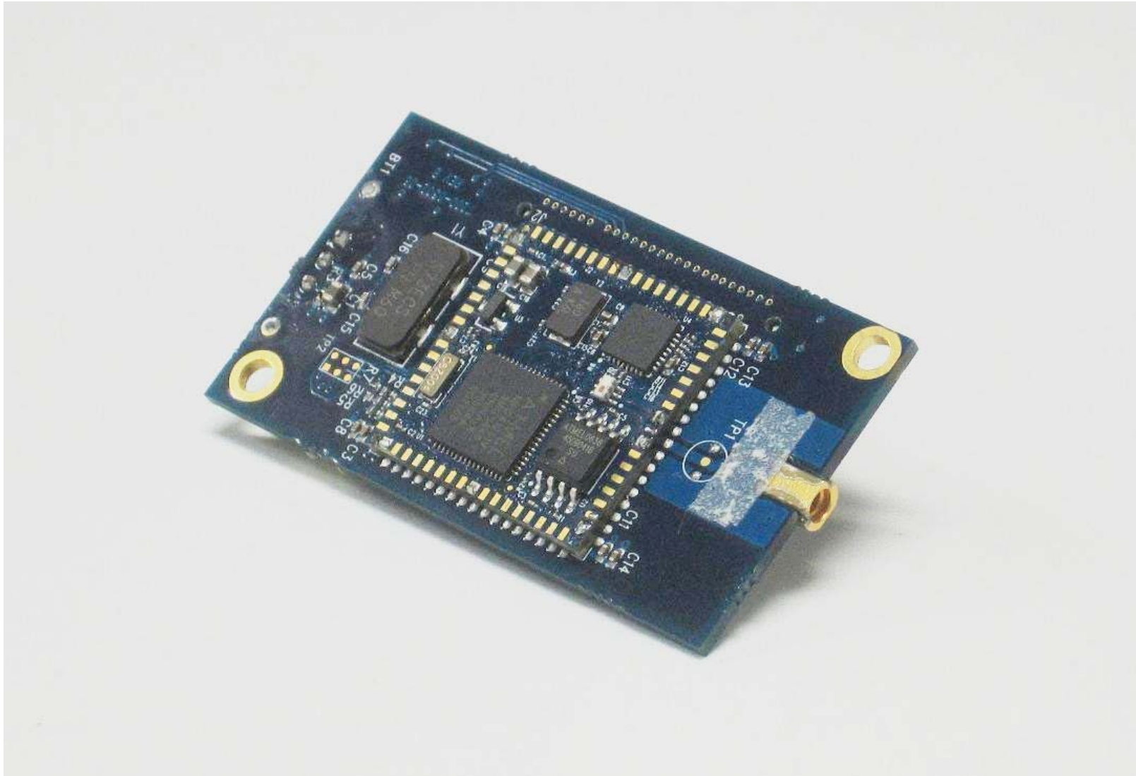
Top side of Radio Board with RF Shield Removed
