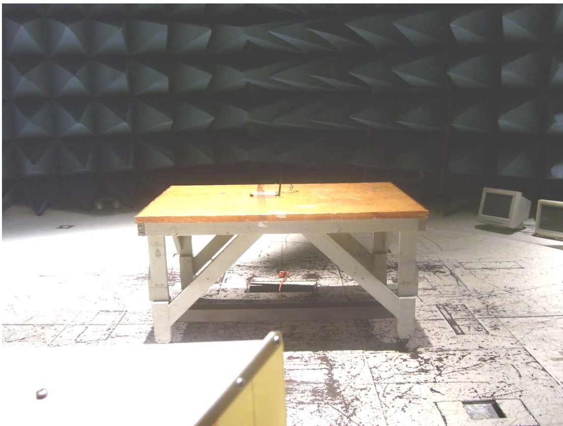
Photograph 3. Test Equipment and setup for various Radiated Measurements
