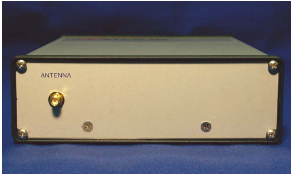
Figure 3 – Reader Rear Panel Showing Antenna Connection
