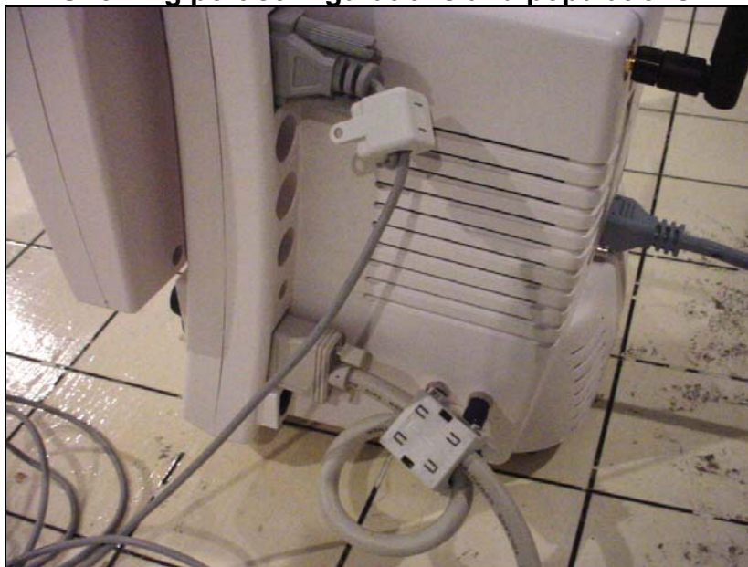
View of the 'Remote' EUT during radiated emissions test, Showing port configurations and populations.
