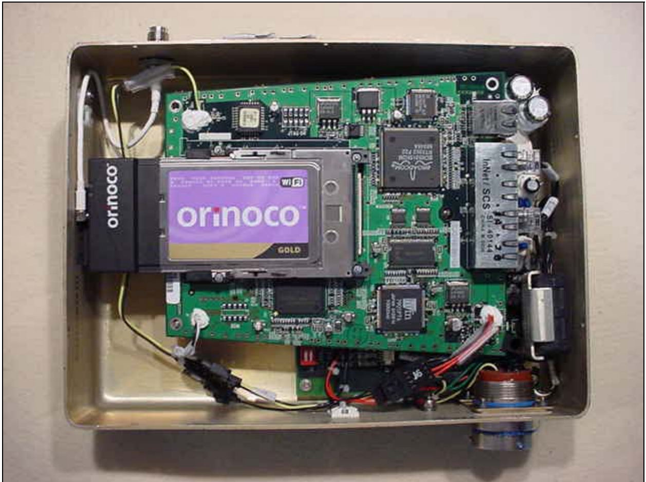
Figure 1: Internal – Cover Removed
