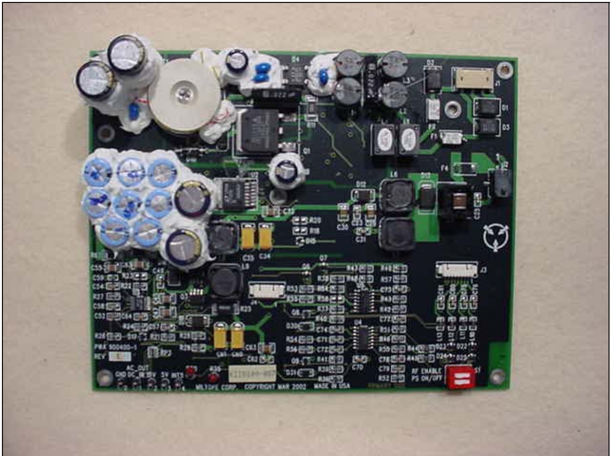
Figure 4: Internal – Power Supply Board (Top View)
