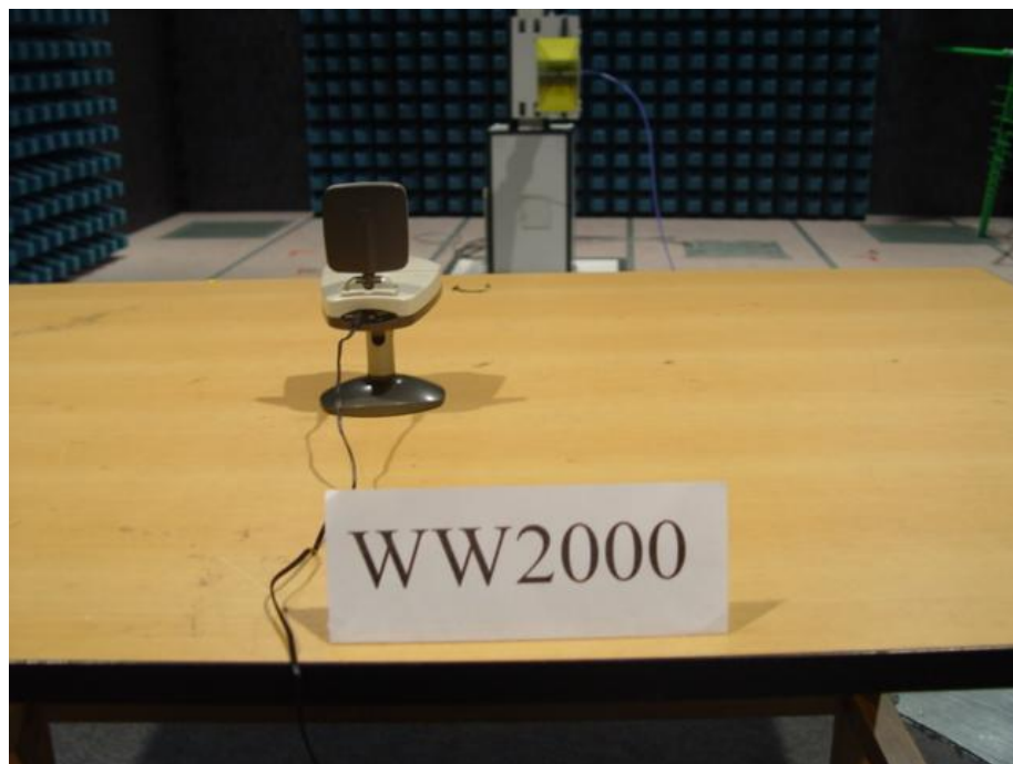
Photo3 Test Setup for Radiated Disturbance Test
