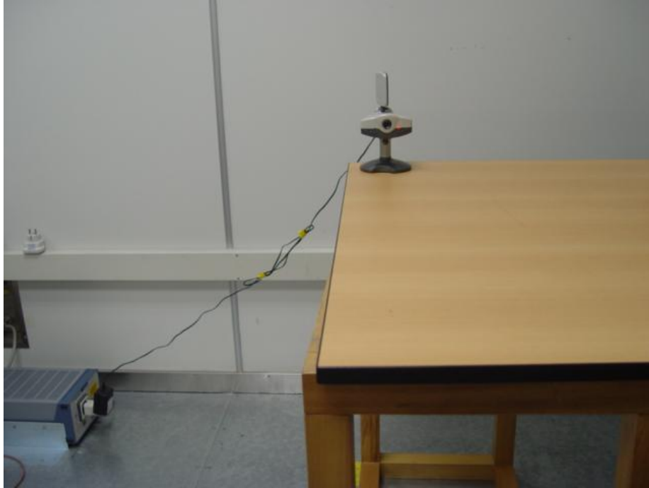
Photo 1 Test Setup for Conducted Disturbance Test
