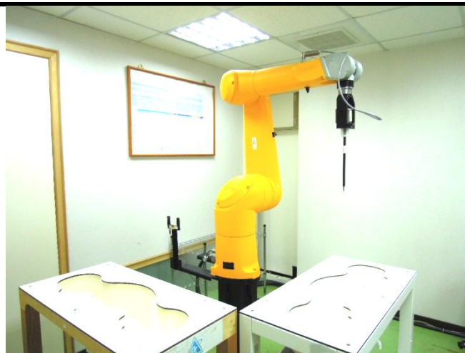
Fig-3.2 SPEAG DASY52 System
