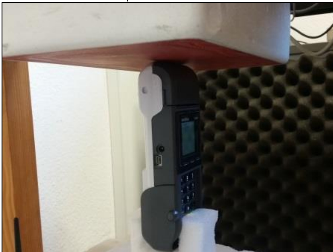
Photo 8: Test position rear side with 0 mm distance
