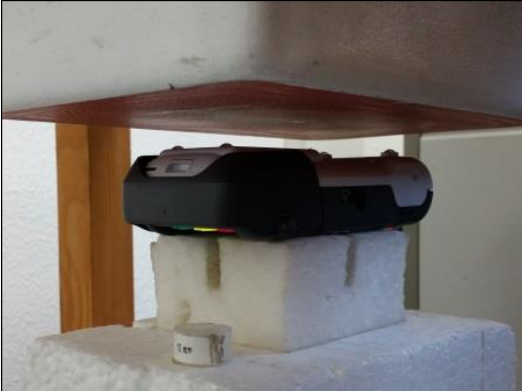
Photo 13: Test position bottom side with 15 mm distance
