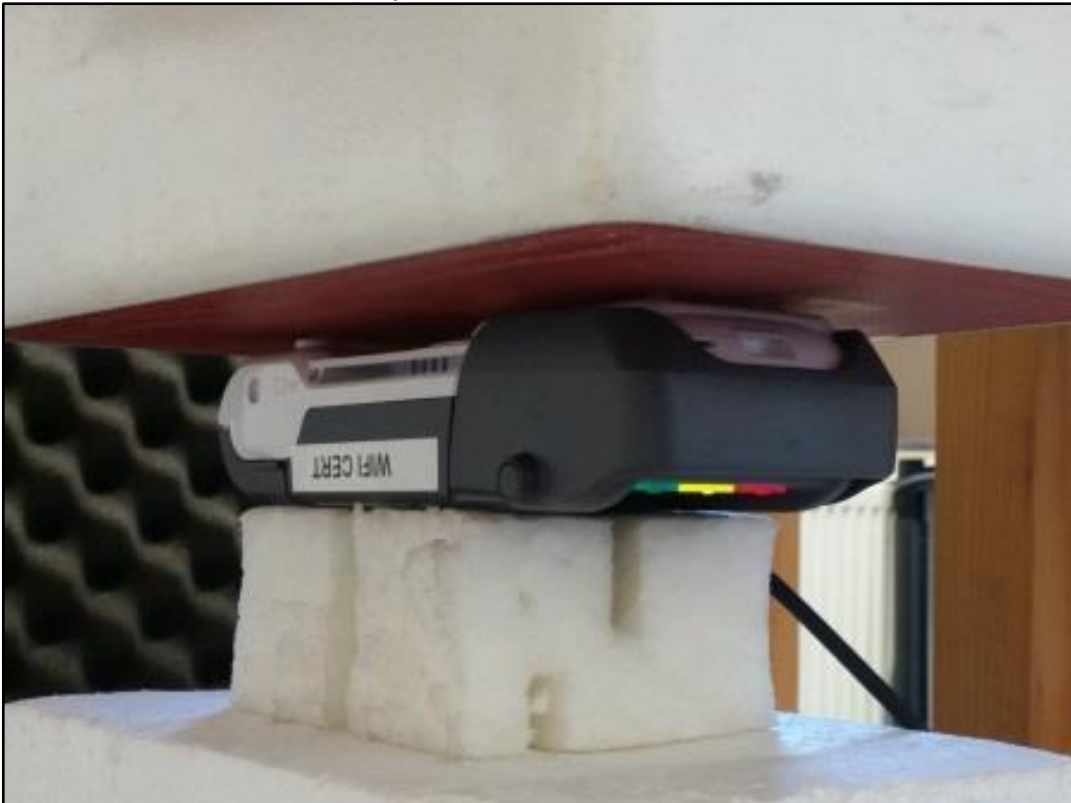
Photo 10: Test position bottom side with 0 mm distance
