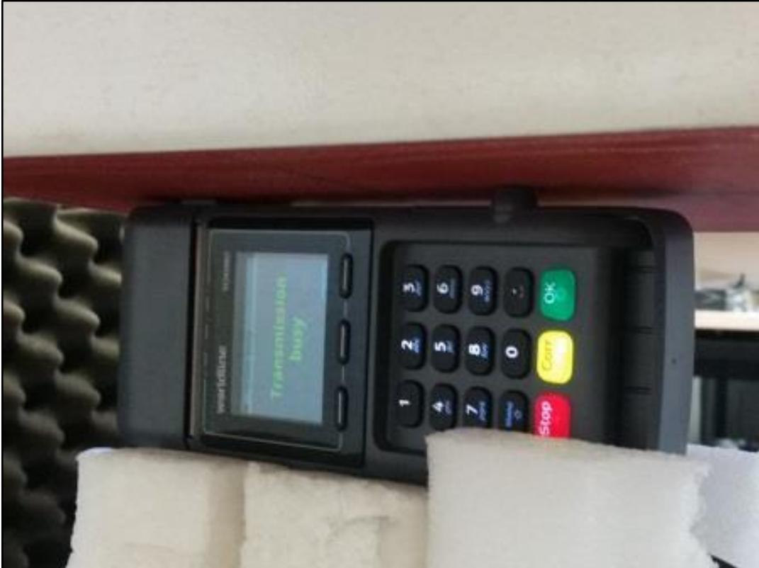
Photo 11: Test position right side with 0 mm distance
