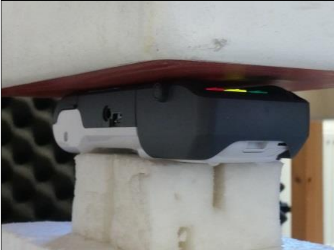
Photo 9: Test position top side with 0 mm distance
