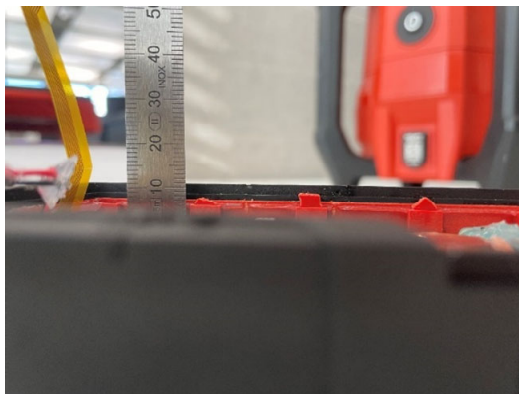
Opened back of the tool without potting material
