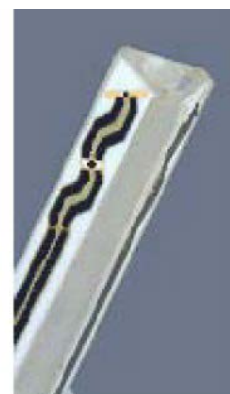
Figure 2.3 Probe Thick-Film Technique
