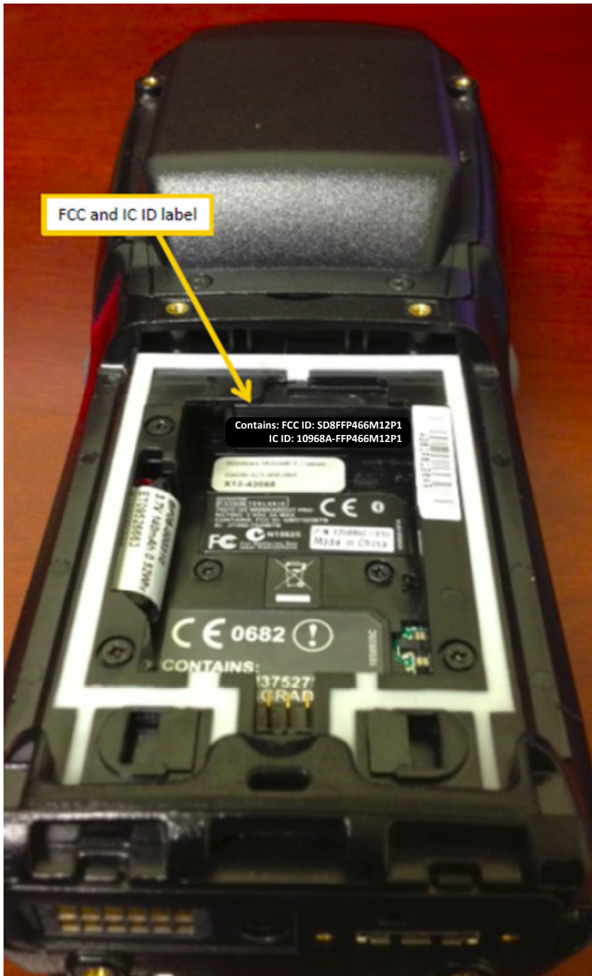
FCC / IC Label and Location beneath the battery compartment of the Host Device.
