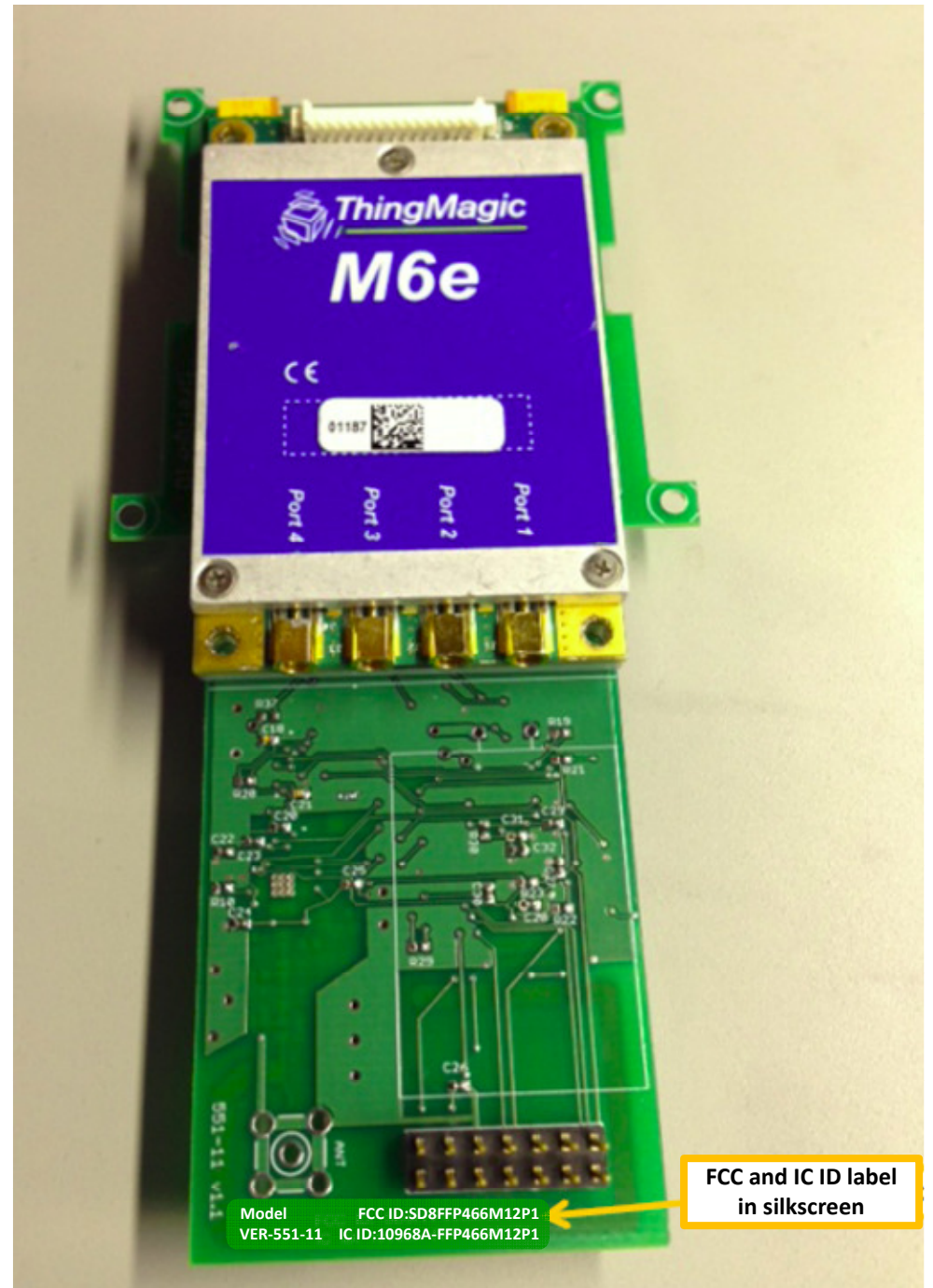
View of FCC / IC Label and Location on the EUT Circuit Board.
