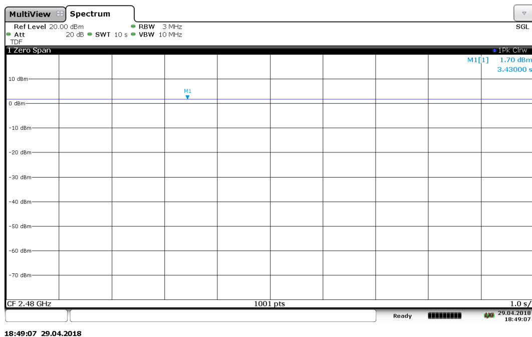
Diagram 23: check of duty-cycle on channel 26 (long 10s period), PWR -4
