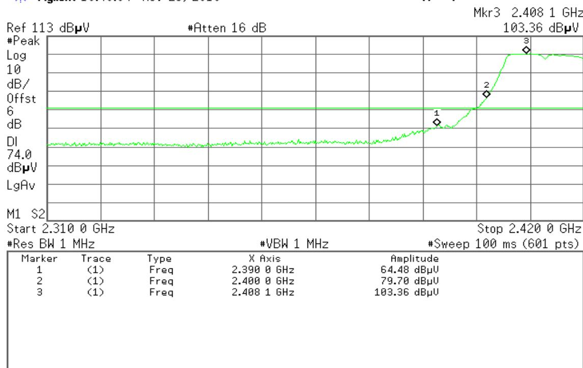
**Detector mode: Average****Polarity: Horizontal****Agilent 16:46:37 Nov 23, 2010**
