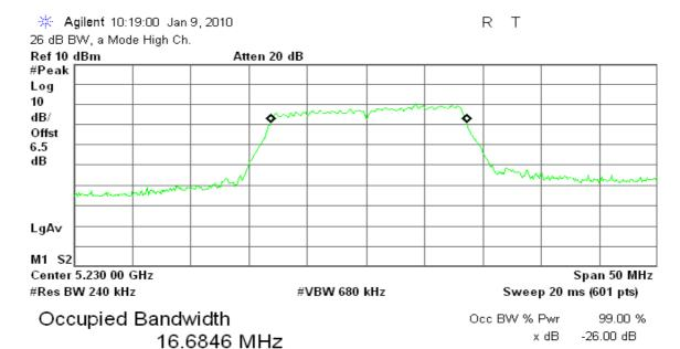
Transmit Freq Error 243.259 kHz x dB Bandwidth 19.785 MHz
