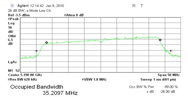
Transmit Freq Error 867.580 kHz x dB Bandwidth 39.502 MHz
