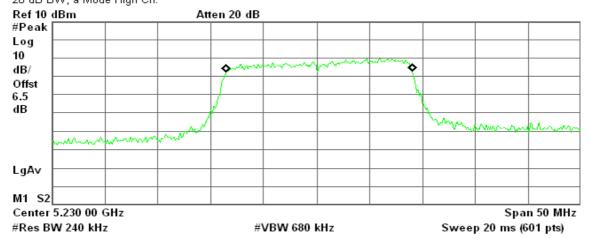
Occupied Bandwidth 17.4670 MHz Occ BW % Pwr 99.00 % x dB -26.00 dB
