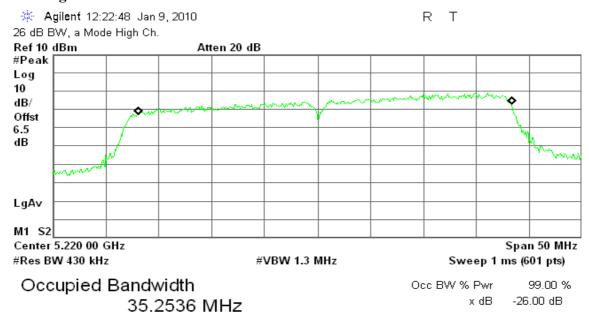
Transmit Freq Error 671.257 kHz x dB Bandwidth 39.087 MHz
