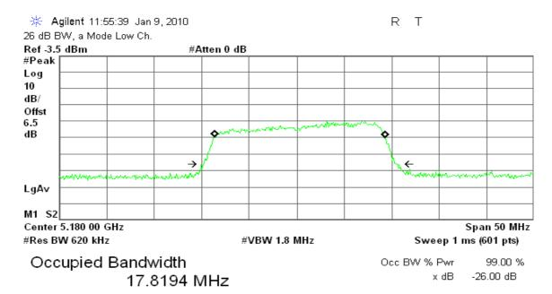
Transmit Freq Error 329.107 kHz x dB Bandwidth 20.259 MHz
