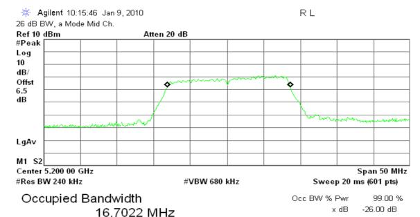
Transmit Freq Error 246.109 kHz x dB Bandwidth 19.866 MHz
