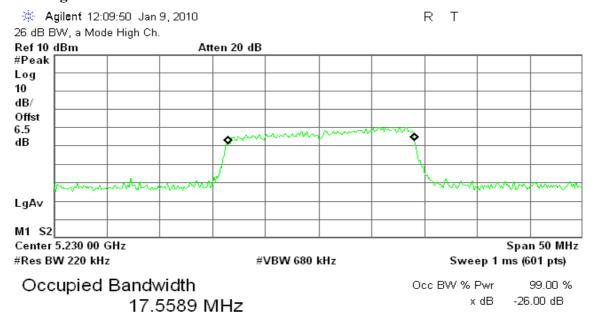
Transmit Freq Error 240.031 kHz x dB Bandwidth 19.448 MHz
