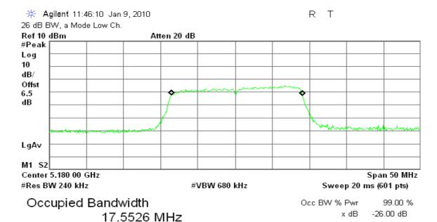
Transmit Freq Error 245.709 kHz x dB Bandwidth 20.219 MHz
