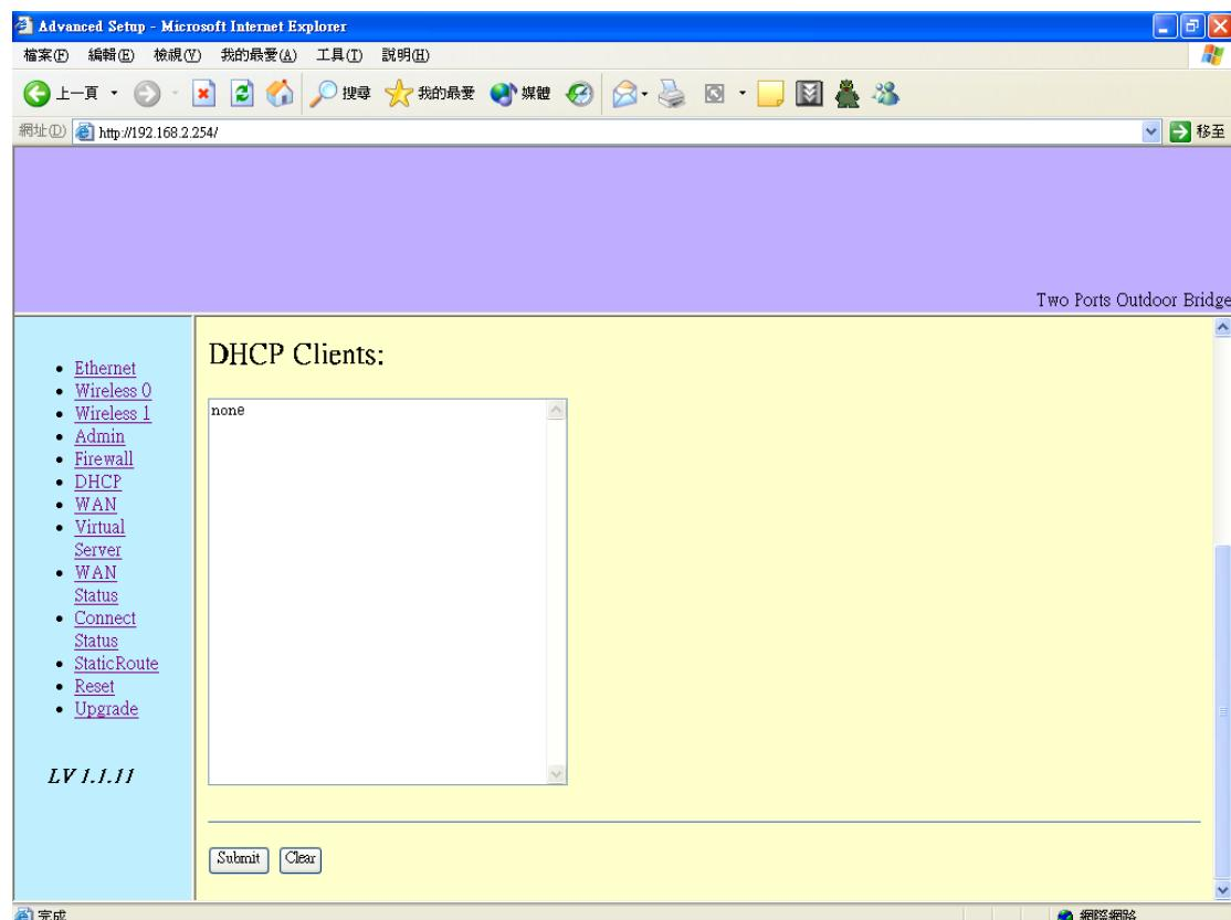
**DHCP Server Control: Dynamic Host Configuration Protocol** assigns dynamic IP addresses to devices on the network. This protocol simplifies network management and allows new wireless devices to receive IP
