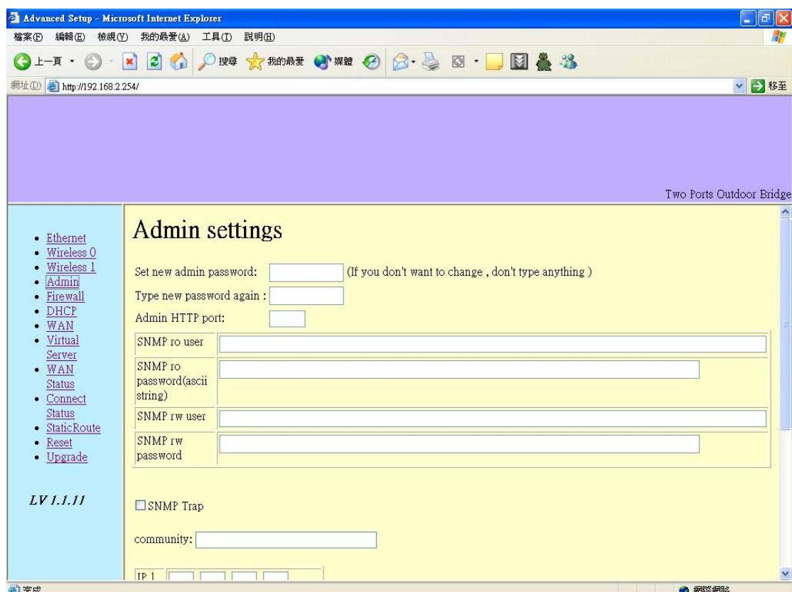
You can change login password (default password is “**default**”), SNMP user name and password, and SNMP Trap setting here.
