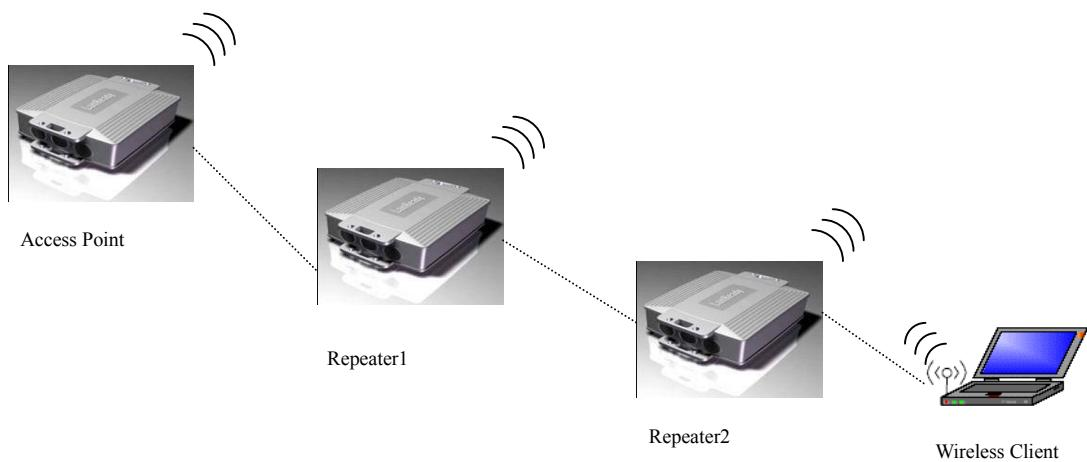
Repeater mode setting is like AP mode setting, but encryption only WEP encryption method can select.
