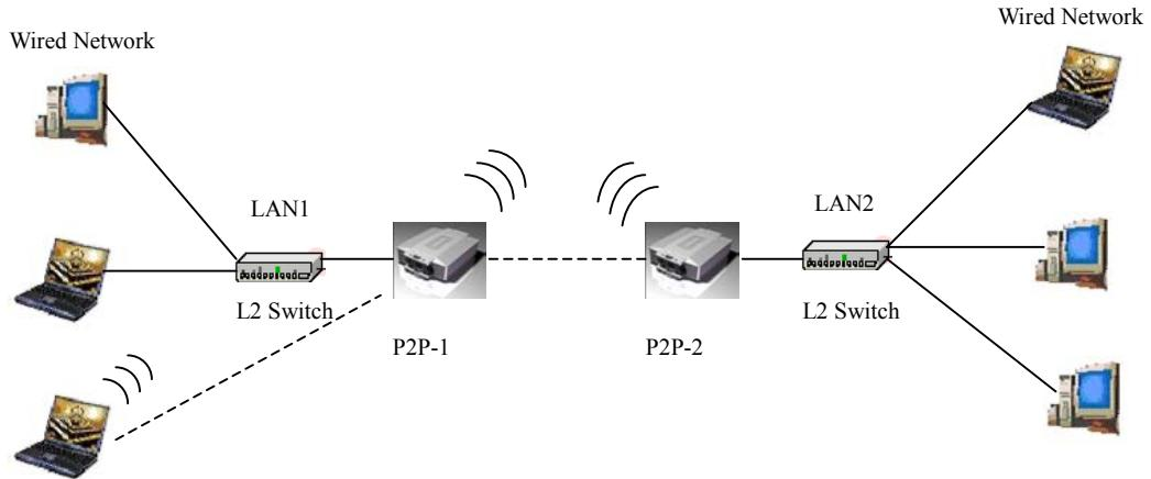
PtP mode setting is like AP mode setting, but encryption only WEP encryption method can select. When wireless0 or wireless1 in PtP mode will also do AP function, suggest disable SSID broadcast(Pull down select “y” in **hidden SSID** to disable SSID broadcast) and set WEP encryption.
