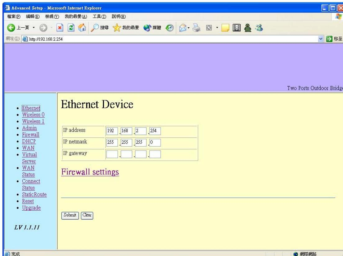
LAN is short for Local Area Network. This is considered your internal network. These are the IP settings of the LAN interface for the OUTDOOR BRIDGE.
