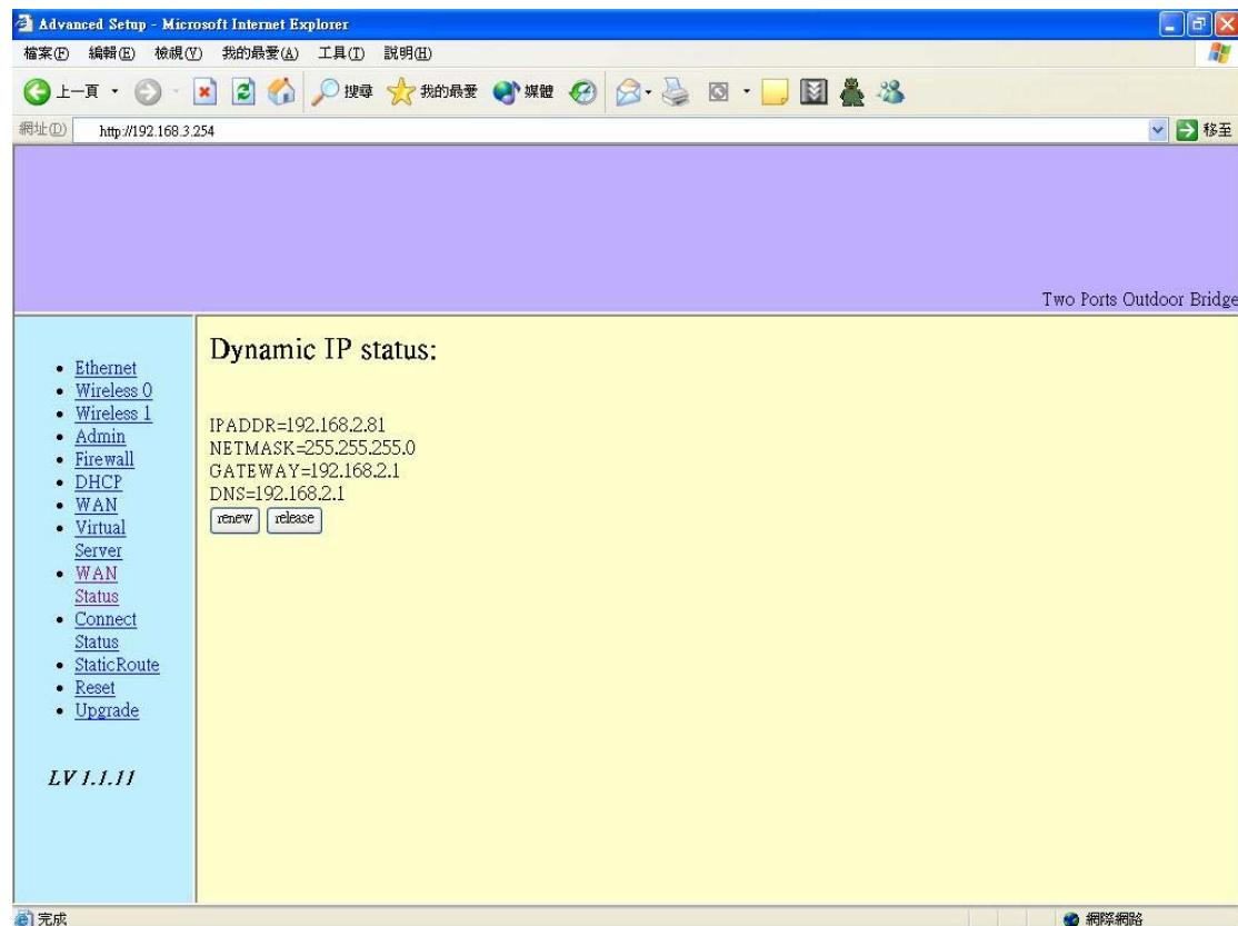
When WAN setting is **Dynamic IP** or **PPPoE** click WAN Status will show current IP status. You can click **renew** or **release** to renew or release IP at **Dynamic IP** setting, and click **disconnect** or **connect** to disconnect or connect your ISP at **PPPoE** setting.
