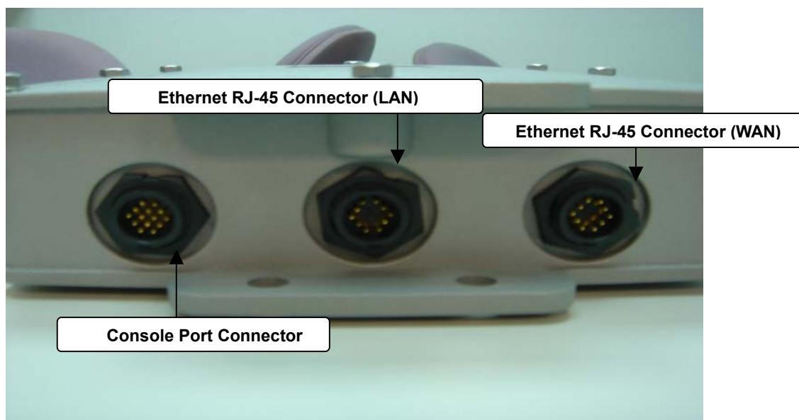
**Console Port** --- It is used for initial setup and configuration of the device
