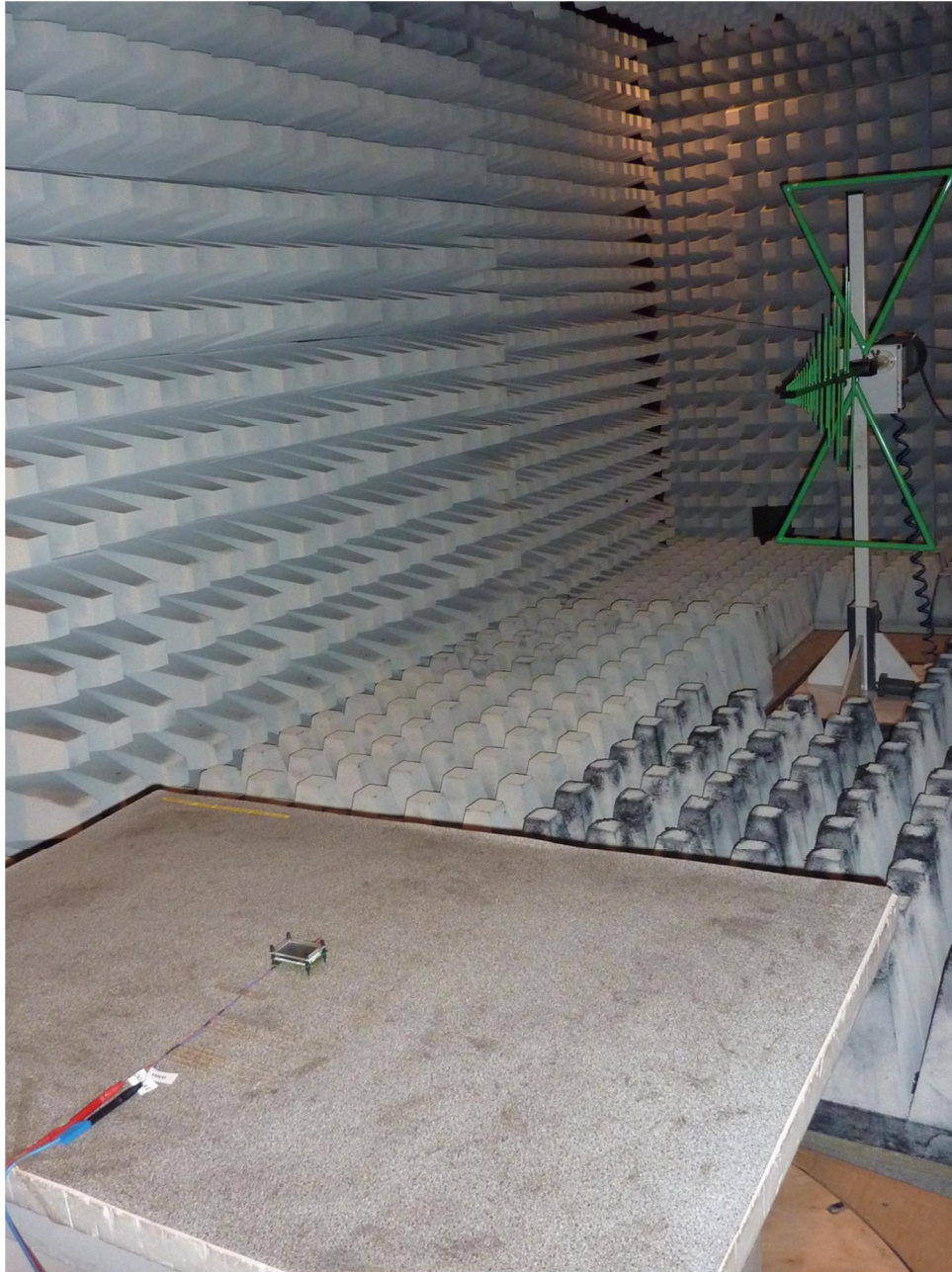
130413_5.JPG: Test setup fully anechoic chamber
