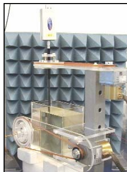
Spherical isotropy jig showing probe
