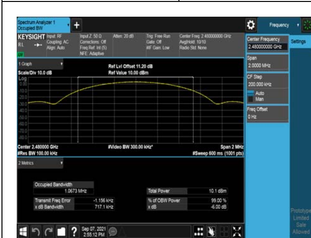
Modulation: 1Mbps 2480MHz
