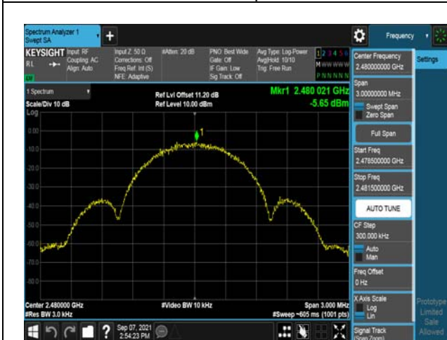
Modulation: 1Mbps 2480MHz
