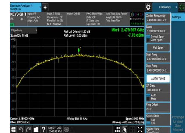
Modulation: 2Mbps 2480MHz
