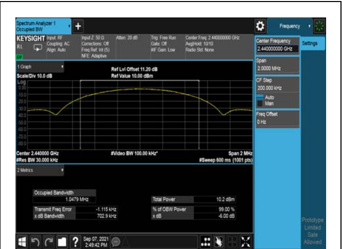
Modulation: 1Mbps 2440MHz
