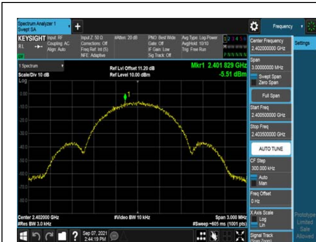
Modulation: 1Mbps 2402MHz
