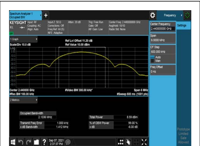
Modulation: 2Mbps 2440MHz
