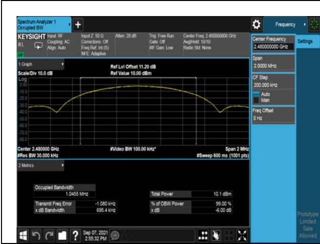
Modulation: 1Mbps 2480MHz
