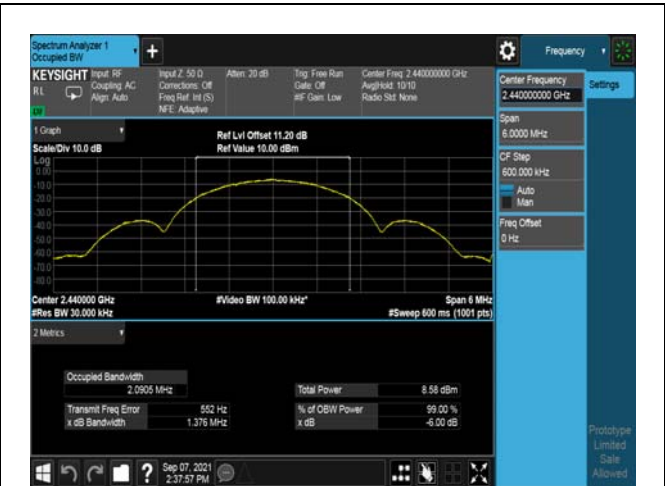
Modulation: 2Mbps 2440MHz
