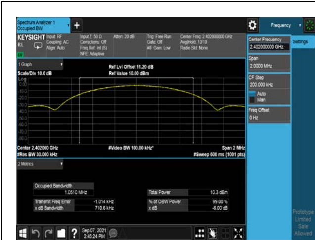
Modulation: 1Mbps 2402MHz
