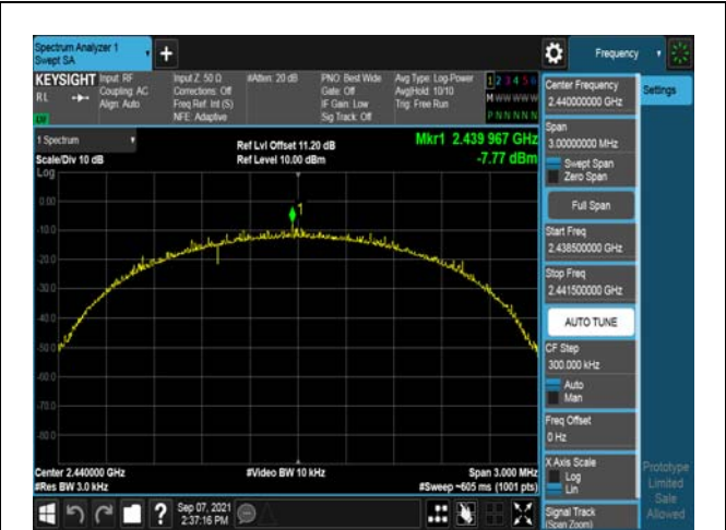
Modulation: 2Mbps 2440MHz
