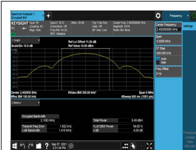
Modulation: 2Mbps 2402MHz
