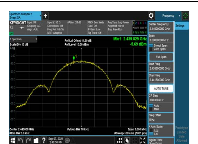
Modulation: 1Mbps 2440MHz
