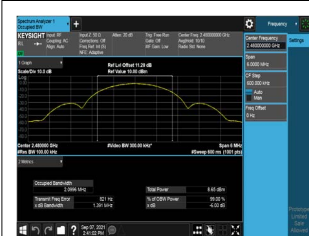
Modulation: 2Mbps 2480MHz
