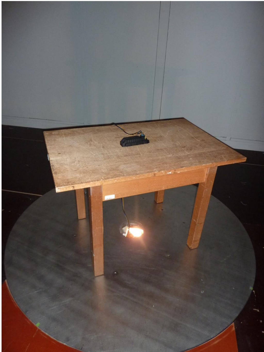
150998_i.JPG: OptiTire ECU, test set-up open area test site, pos. 1
