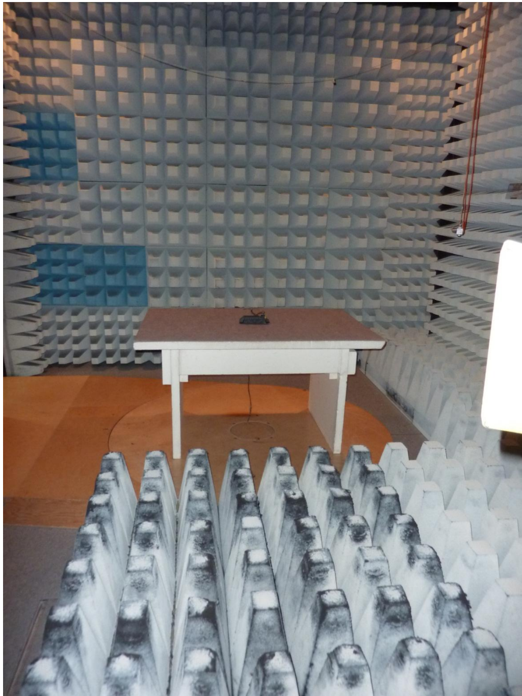
150998_g.JPG: OptiTire ECU, test set-up fully anechoic chamber
