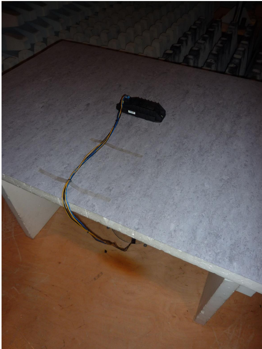
150998_e.JPG: OptiTire ECU, test set-up fully anechoic chamber, pos. 1
