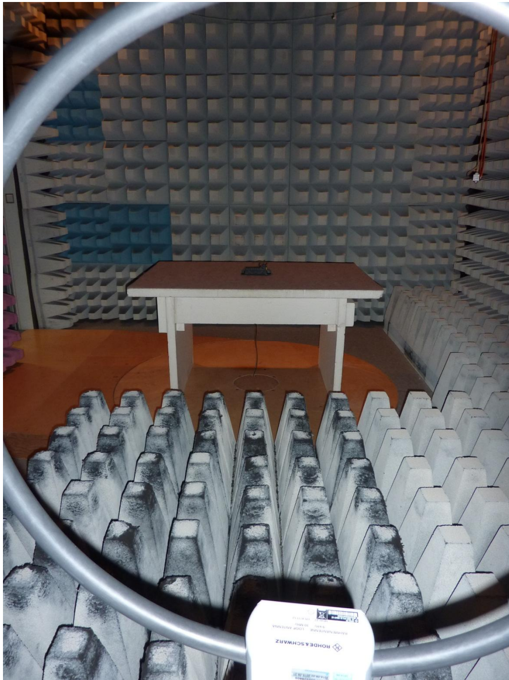
150998_h.JPG: OptiTire ECU, test set-up fully anechoic chamber
