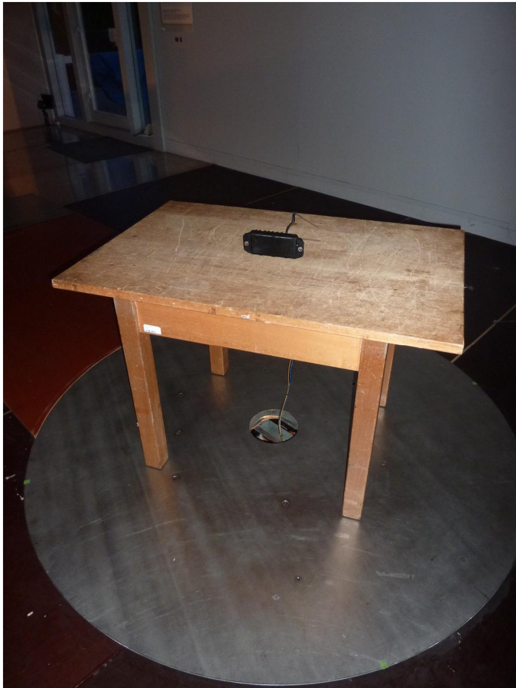
150998_.JPG: OptiTire ECU, test set-up open area test site, pos. 2
