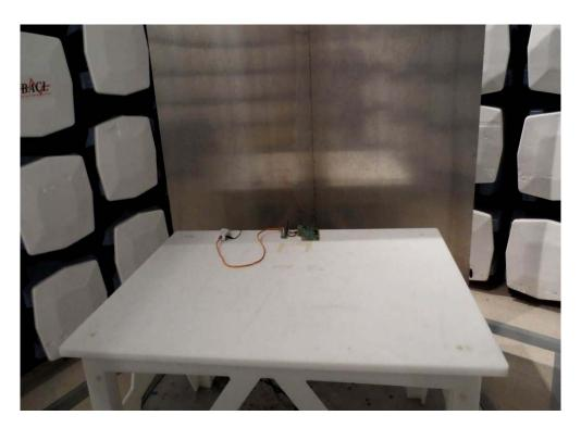
14.6 AC Line Conducted Emission Side View
