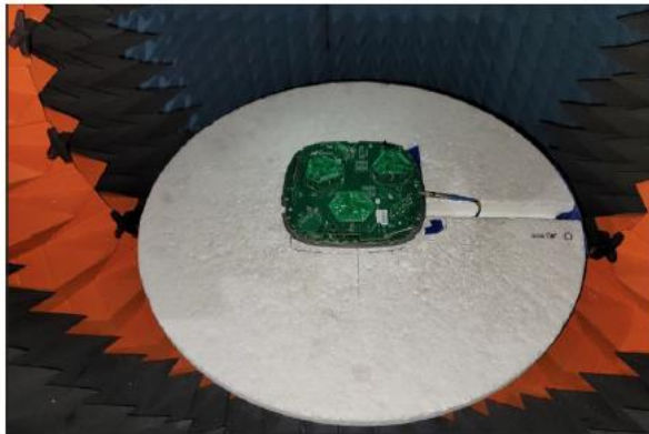
Test setup pictures - MIMO anechoic chamber
