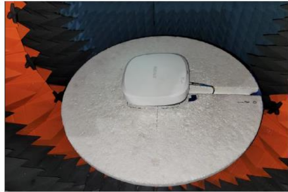
Test setup pictures - MIMO anechoic chamber
