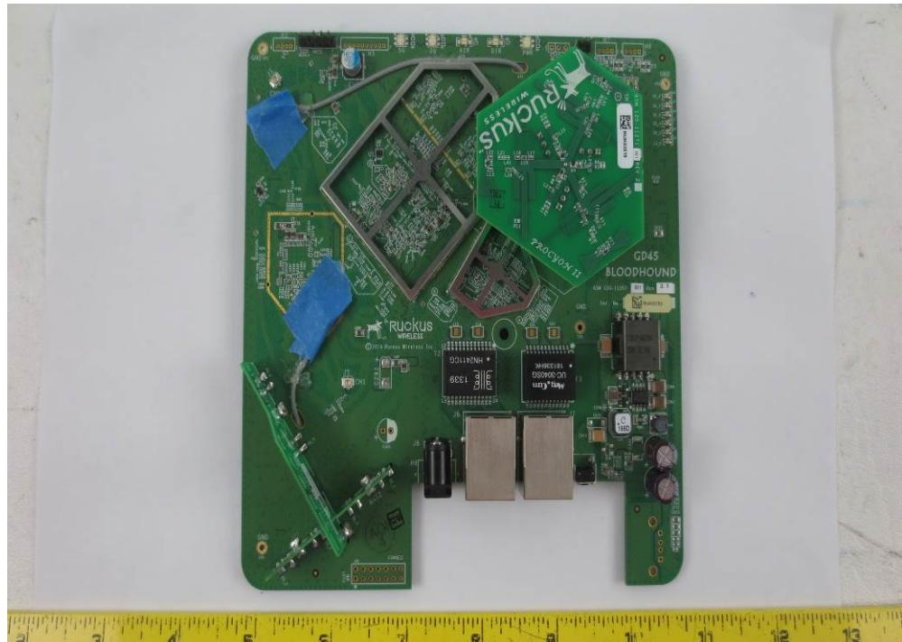
**15.10 PCB Main Board without shielding Bottom View**
