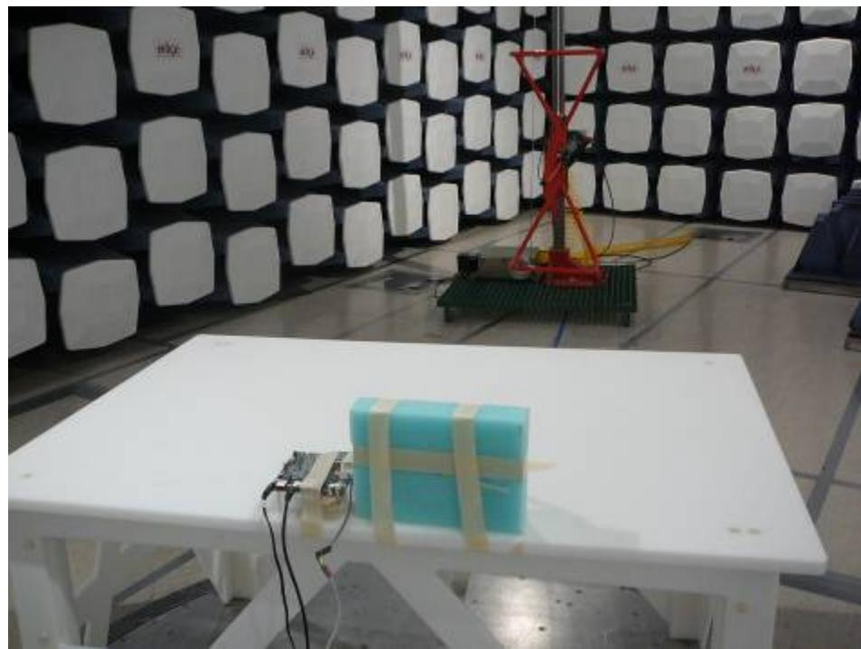
**16.6 Radiated Emission Above 1 GHz Rear View (co-location)**
