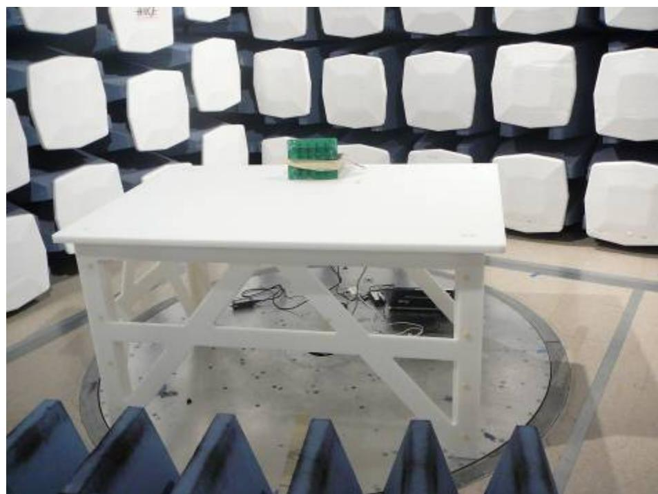
**16.5 Radiated Emission Below 1 GHz Rear View (co-location)**
