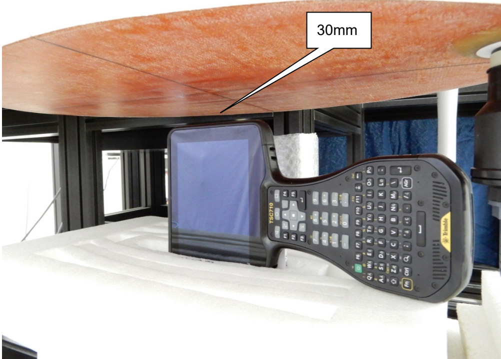
EUT Right-side - 30mm (Antenna 3)
