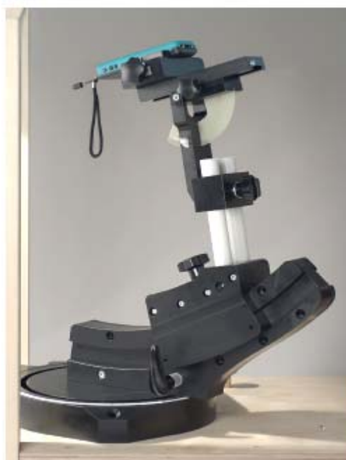
Fig. 10 Device holder supplied by SPEAG
