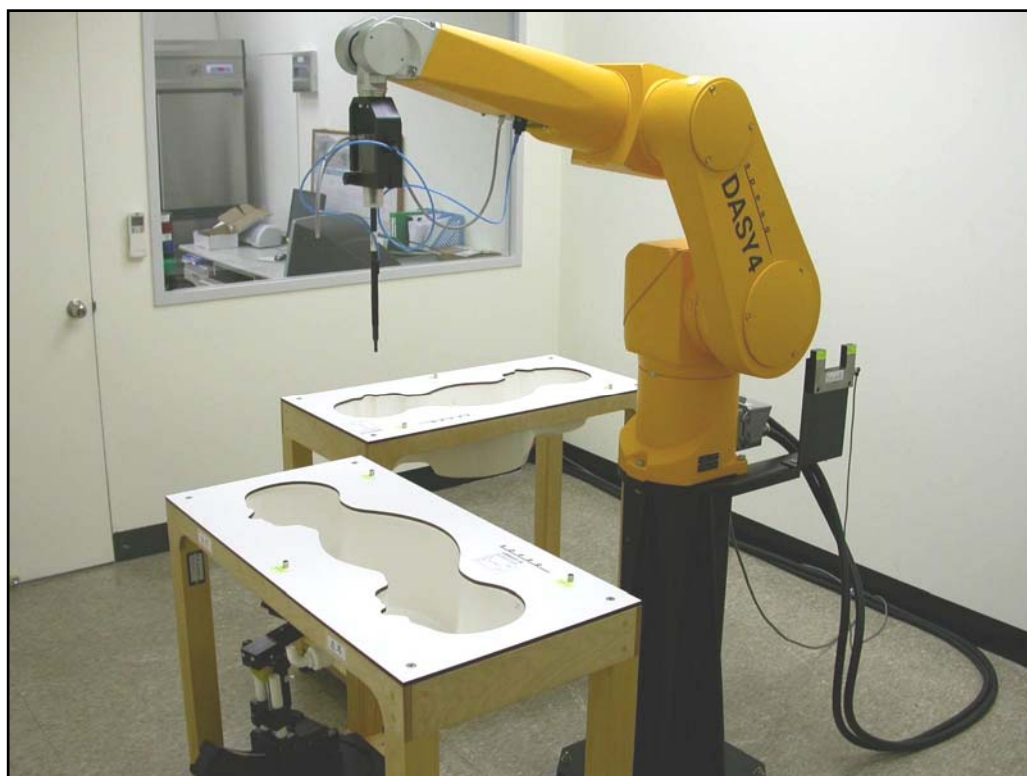
Fig. 6 The DASY4 System used in ETC set-up with two phantoms
