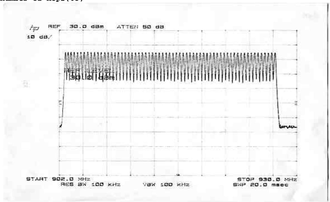
The channel frequency separation(400kHz)
