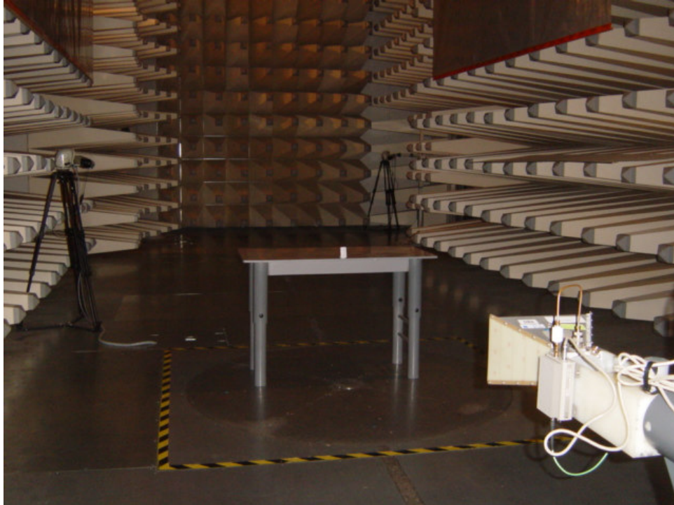
Set up of radiated emission test
