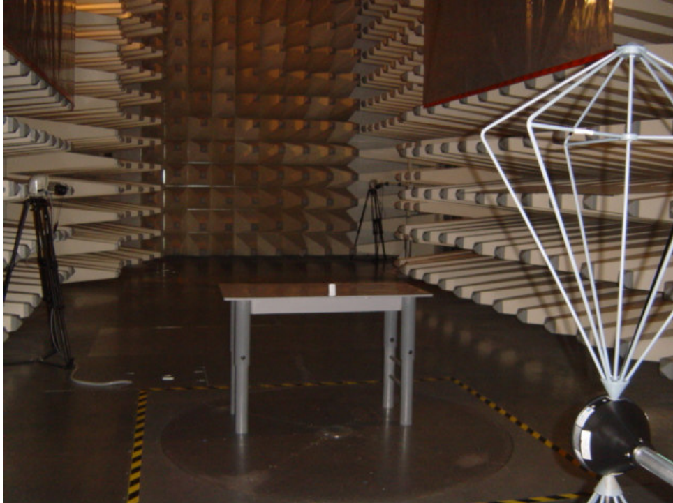
Set up of radiated emission test
