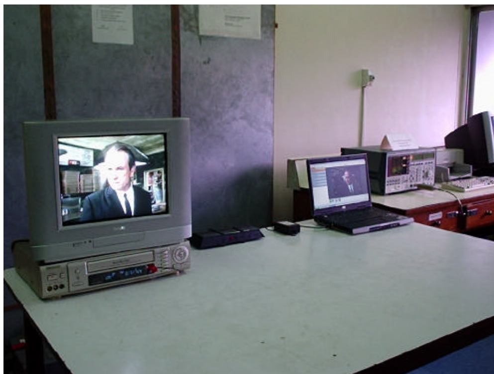
Photograph 1: Set-up for Conducted Emission on AC Mains
