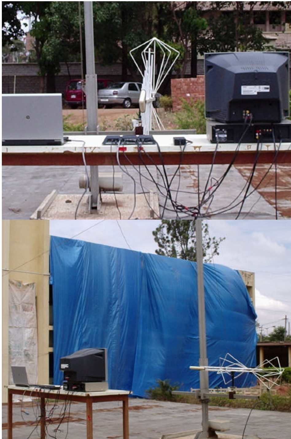
Photograph 3: Set-up for Radiated Emission at OATS
