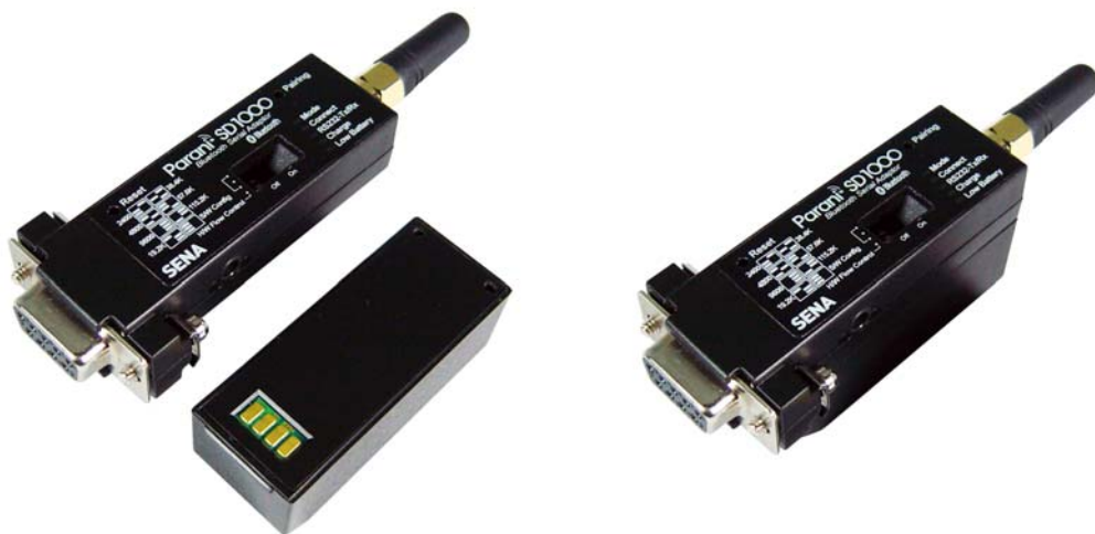
Figure 2-4 Attaching Battery Pack to Parani-SD1000
