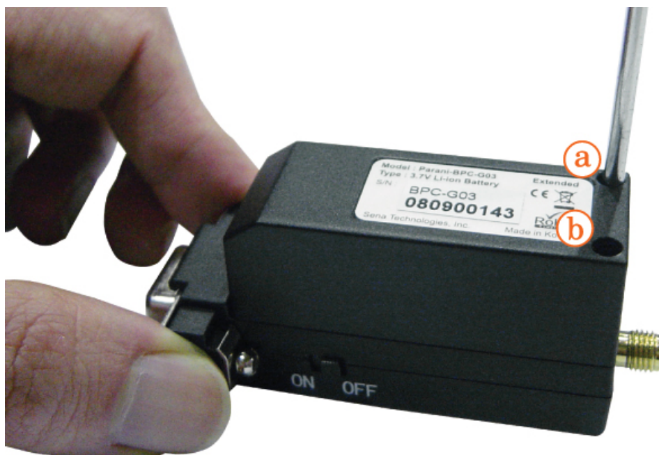
Figure 2-7 Fasten the battery pack
