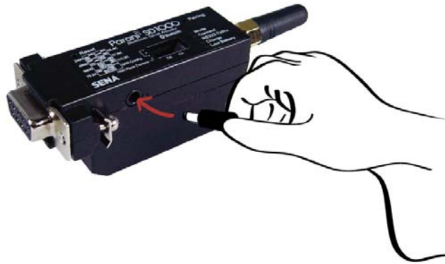
Figure 2-2 Connecting Power to Parani-SD1000
