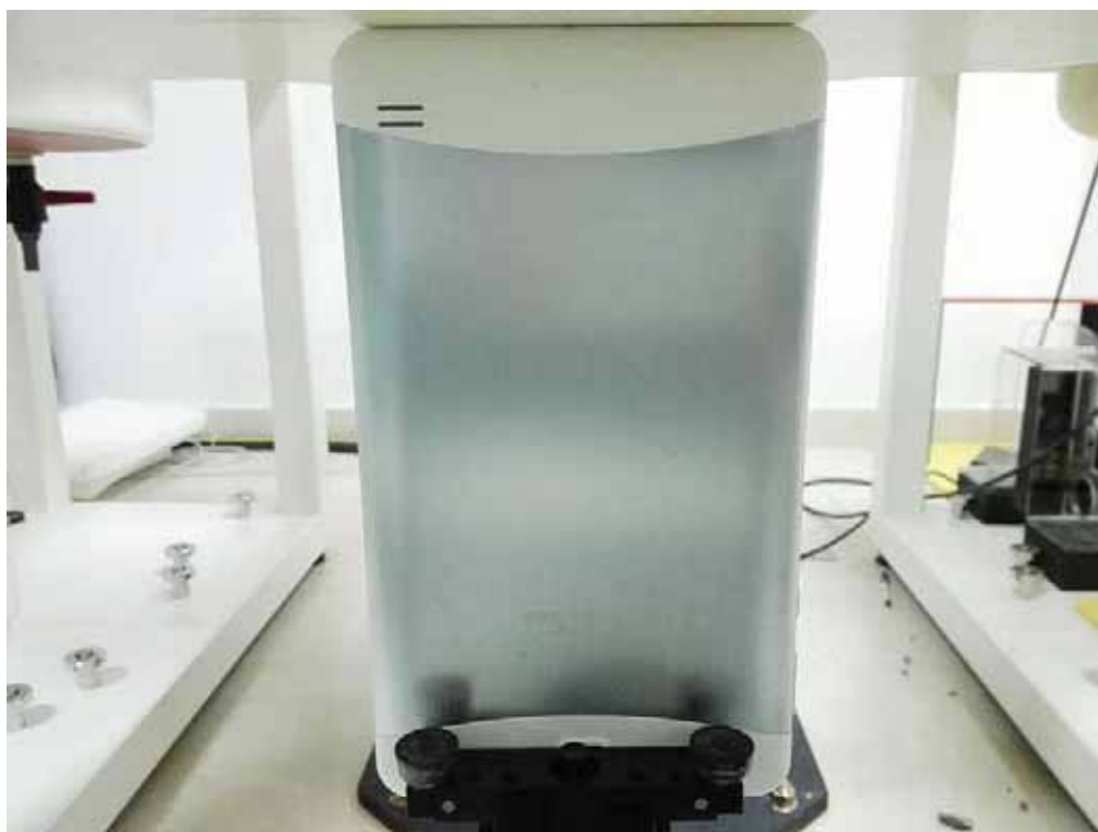
0mm Body-worn Bottom Side Setup Photo
