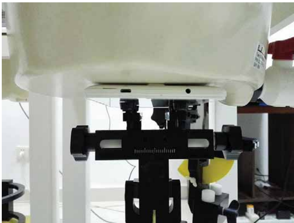
0mm Body-worn Rear Side Setup Photo
