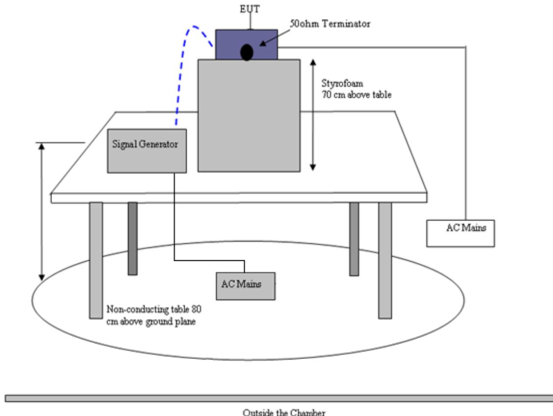
Note: For radiated emissions measurements performed at frequencies less than or equal to 1 GHz, the EUT shall be placed on the Non-conducting table at a nominal height of 80 cm above the reference ground plane.
