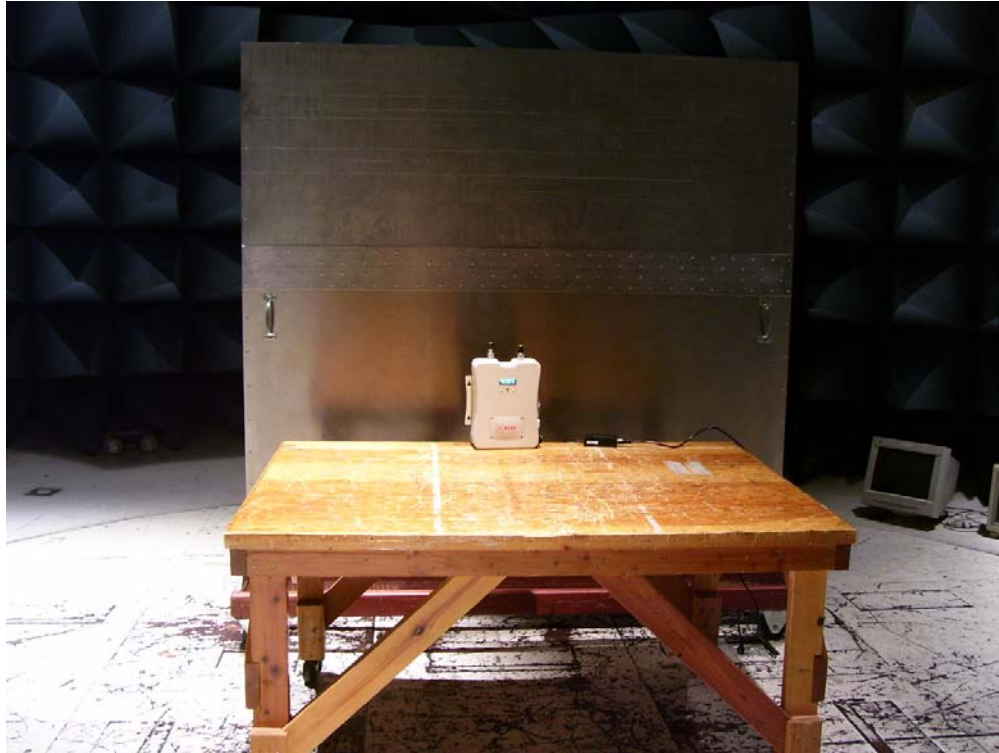
Photograph 2. Conducted Emissions Test Setup, Front View
