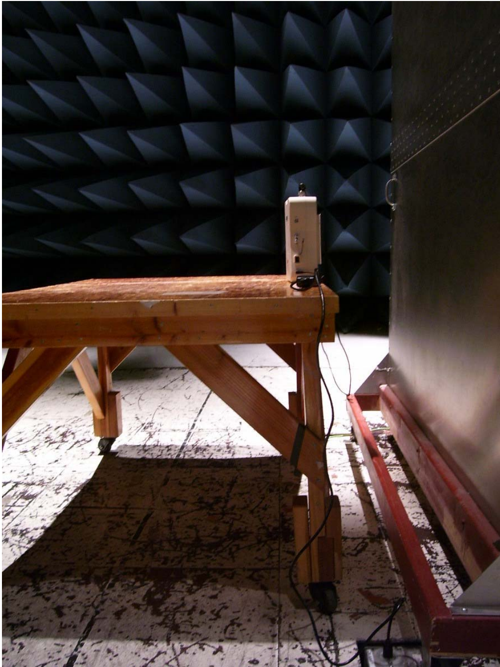
Photograph 3. Conducted Emissions Test Setup, Back View
