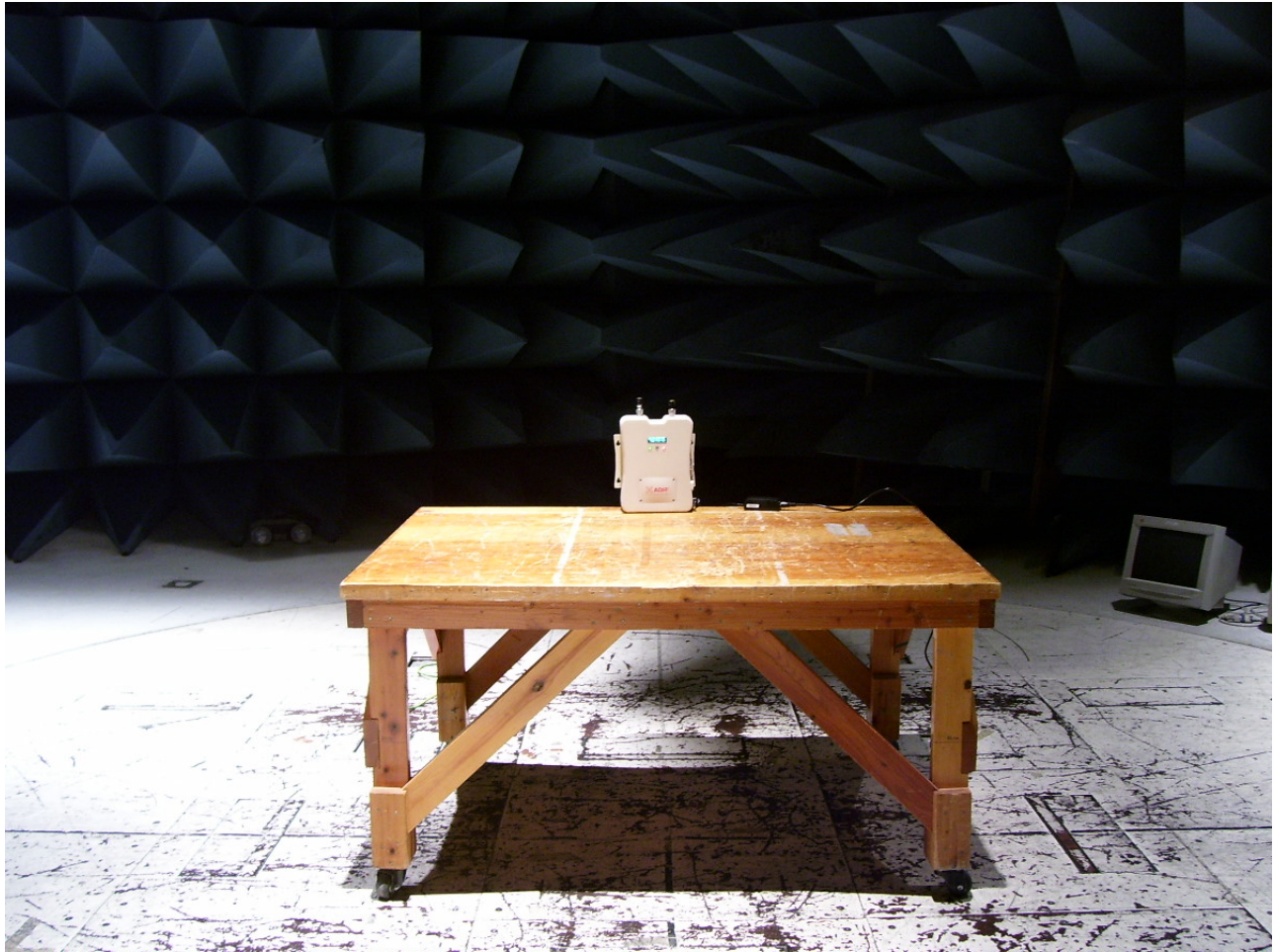
Photograph 4. Radiated Emission Limits Test Setup
