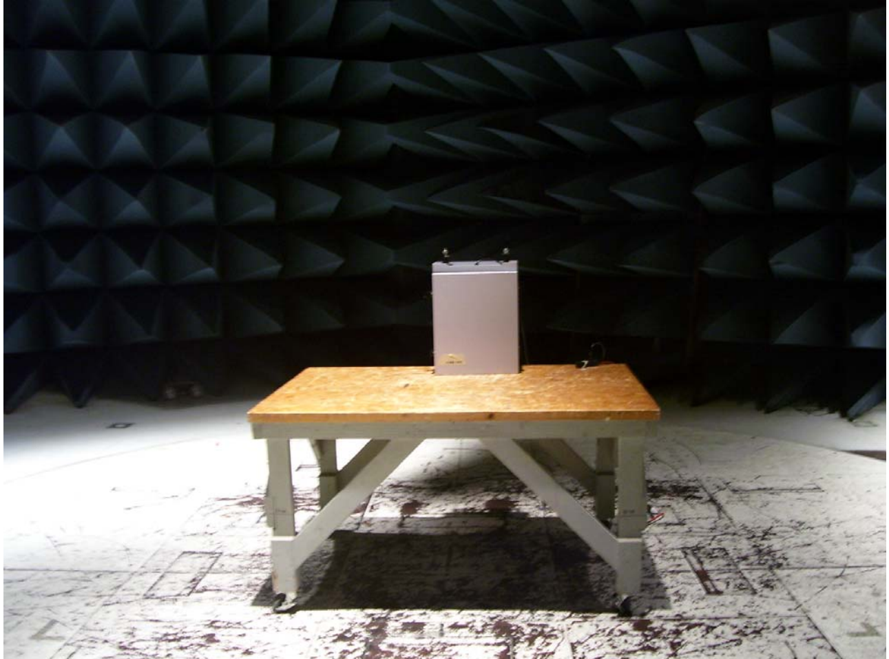
Photograph 3. Radiated Emission Limits Test Setup
