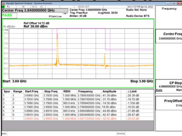
Band77-Part27_100MHz_DFT_s_OFDM_SCS30kHz_BPSK_RB1_0_CH626000
