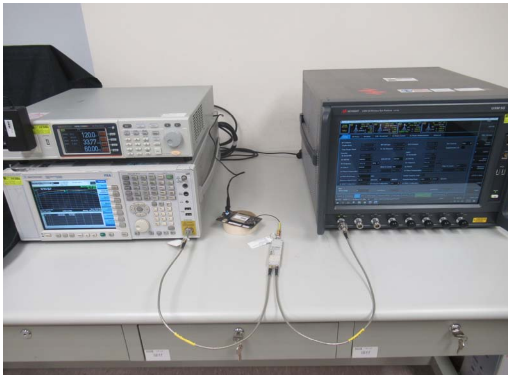
Conducted Setup Photo (Measurement at Antenna Port)
