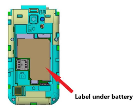
The batteries are designed for easy removal and the label will be visible whenever the batteries are removed for charging or replacement.
