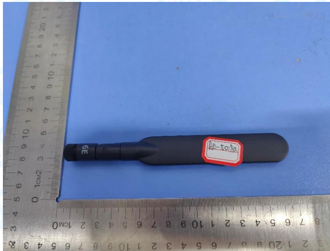
Antenna 7: 3.52dBi Dipole Antenna(AD-510AX)
