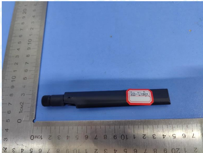
Antenna 8: 3.02dBi Dipole Antenna(AD-512AX)
