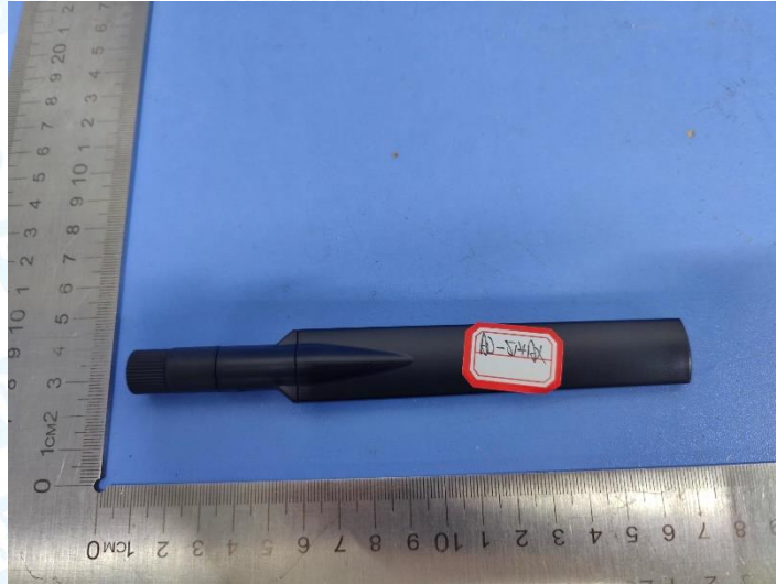
Antenna 10: 6.34dBi Dipole Antenna(AD-515AX)
