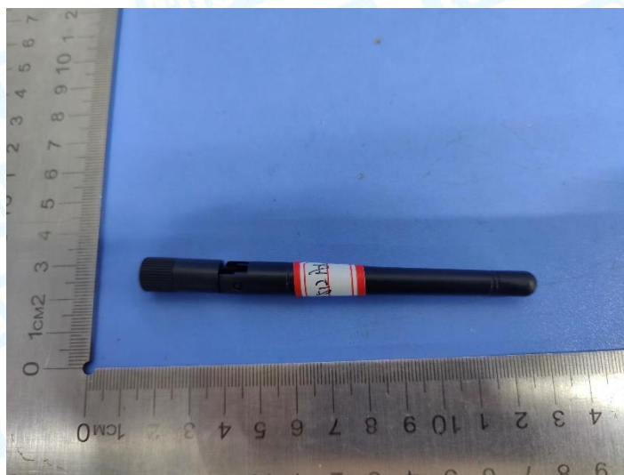
Antenna 8: 3.02dBi Dipole Antenna(AD-512AX)
