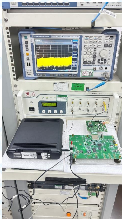
Photo of Setup for DFS Test
