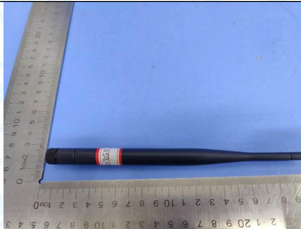
Antenna 6: 5.0dBi Dipole Antenna(AD-501AX)
