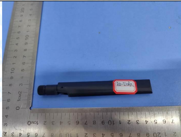
Antenna 8: 3.02dBi Dipole Antenna(AD-512AX)
