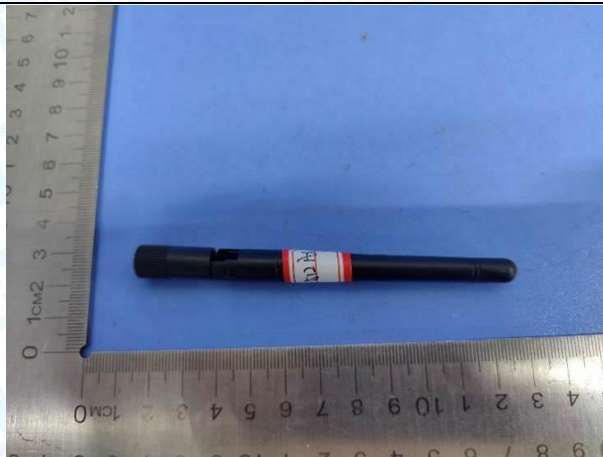
Antenna 9: 4.17dBi Dipole Antenna(AD-514AX)
