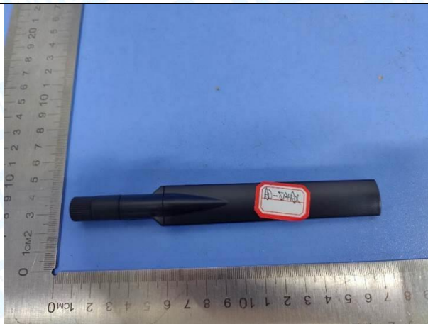
Antenna 9: 4.17dBi Dipole Antenna(AD-514AX)
