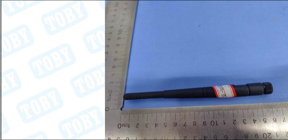
Antenna 2: 5.8dBi Dipole Antenna(AD-301N)
