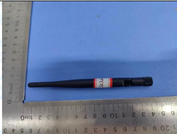
Antenna 5: 5.53dBi Dipole Antenna(AD-305N)
