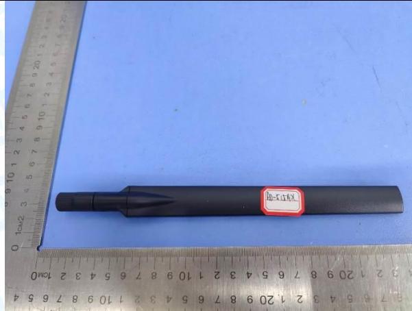
Antenna 10: 6.34dBi Dipole Antenna(AD-515AX)
