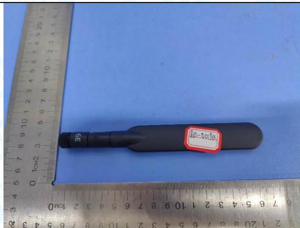
Antenna 6: 5.0dBi Dipole Antenna(AD-501AX)
